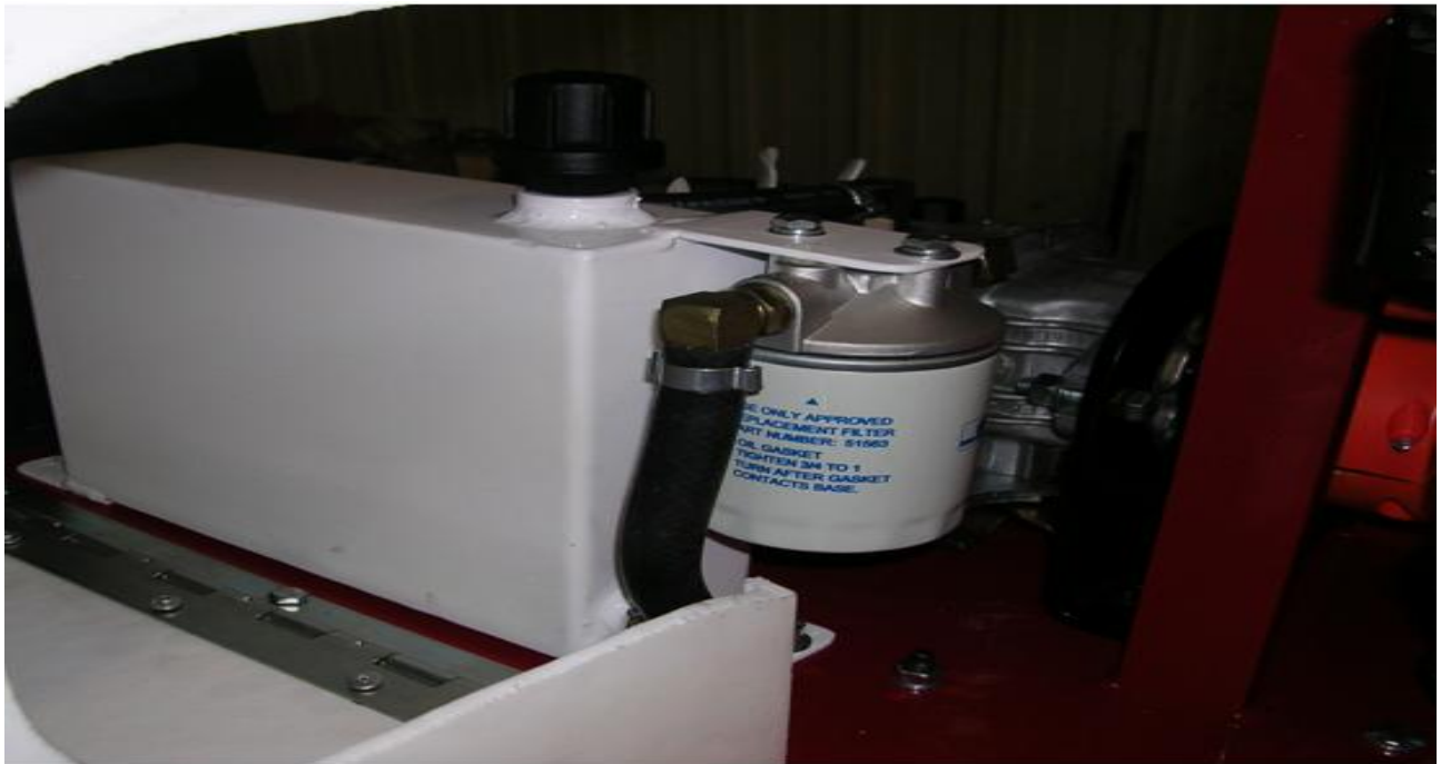
greensIRON Pump Reservoir and Filter
